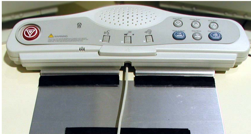
Figure 2-10 SCIM control with keyboard cable routed through SCIM
