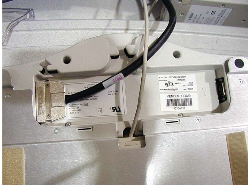
Figure 2-11 SCIM bottom, showing cables and keyboard mounting bracket
