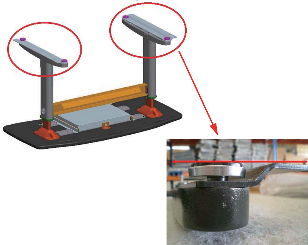
Figure 12 Installation Direction of Anti Seismic Brackets
