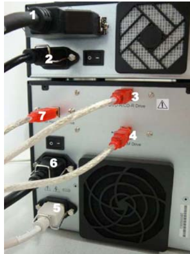
Figure 2-12 Media Tower Connections shown with optional MOD Drive
